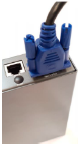
Connect the monitor to the VGA port
