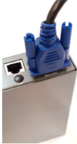
Connect the monitor to the VGA port
